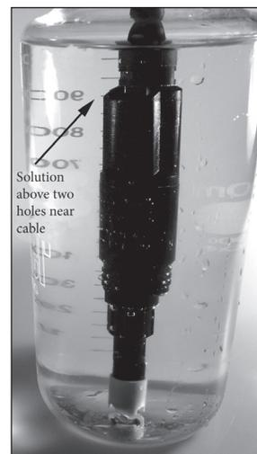
Figure 8, solution above two holes near cable.
