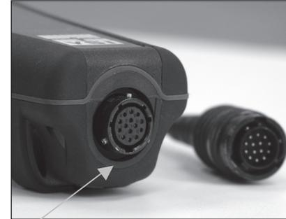
Figure 4, Note the keyed connector.
